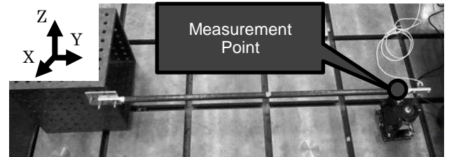
Length:1090[mm] Outer diameter:20[mm] inside diameter:16[mm]
